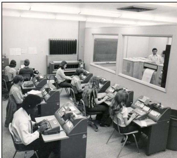
Students in computer class using IBM 026 keypunch machines with the printer and mainframe behind the glass window (ca. 1970). Reproduced by permission, Arizona Memory Project.
