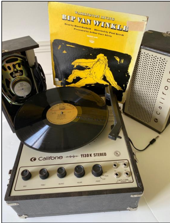
Through a grant from the Maryland State Department of Education, the DSW had Califone record-players (turntables) with three speeds (33 1/2, 45, 78 rpm), detachable stereo speakers, and tone quality adjustment knobs.
